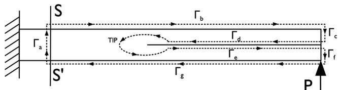
Figure 1.- Integration paths considered in the C-ELS test.
