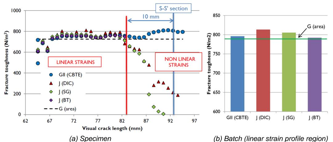
Figure 4.- Fracture toughness obtained from the LEFM ( $G_{II}$ ) data reduction methods and J-integral.
