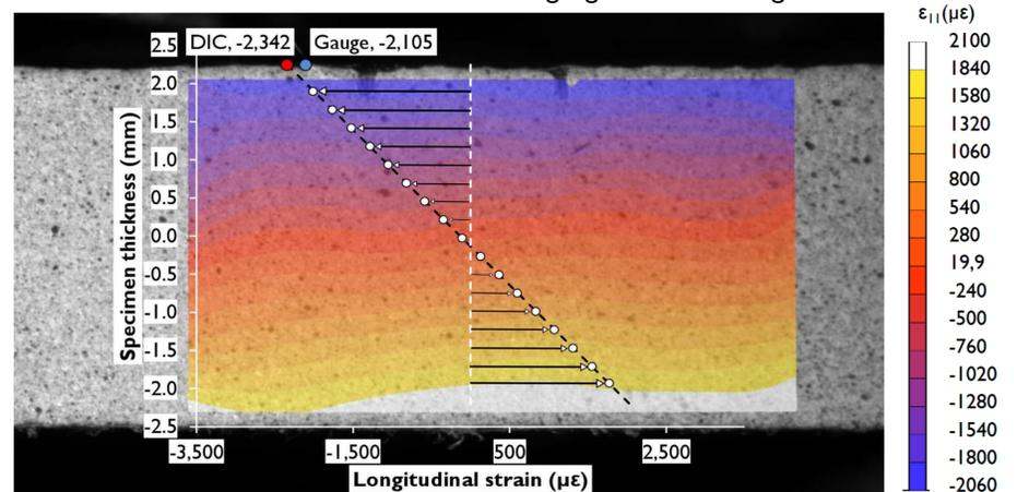
Figure 3.- Strain profile measured at S-S' with DIC (Face B) and the strain gauge.
